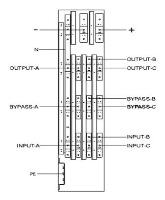
Figure 2-20 8-slot cabinet UPS connection terminals
