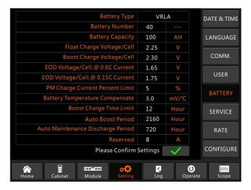
Figure 4-4 setting the period for battery auto discharge
