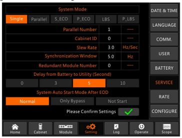
Figure 3-17 the setting interface of SERVICE
