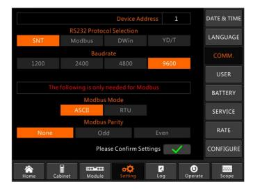
Figure 3-13 the setting interface of COMMUNICATION
