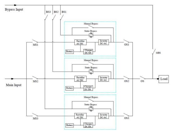
First turn off the battery switch used with the first UPS, and then turn off BS1 and MS1 one by one, and finally turn off OS1, the first UPS will be off. If recover, please first turn on OS1, and then turn on BS1 and MS1 one by one and finally turn on the battery switch.
