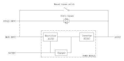
(b) 4-slot and 6-slot UPS Block Diagram
