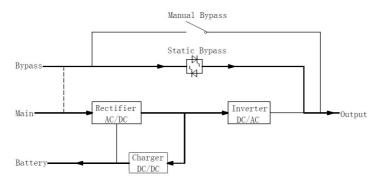
Figure 1-9 ECO Mode operation diagram
