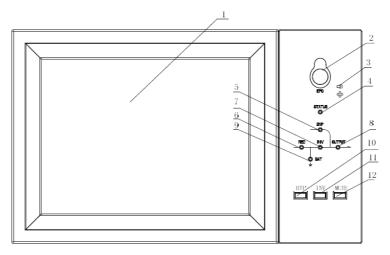
1: LCD touch screen 2: EPO switch 3: Audible Alarm (Buzzer)
