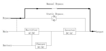
Figure 1-8 Maintenance mode operation diagram
