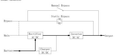
Figure 1-6 Battery Mode operation diagram
