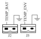
Figure 2-23 J2 and J3 for temperature detecting Table 2-8 Description of J2 and J3
