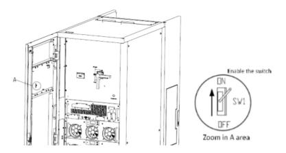
Figure 4-2 enabling the switch
