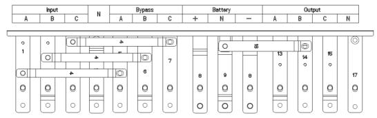
Figure 2-17 2-slot cabinet UPS connection terminals
