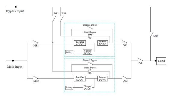
The cable connection drawing for 2 UPSs in parallel (dual input)
