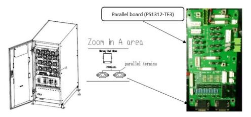
(a) Parallel interface location for 2-slot and 4-slot cabinet (take 4-slot cabinet for example)
