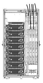
Figure 2-13 Cable Entry for 8-slot cabinet
