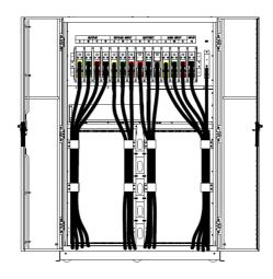
Figure 2-16 Cable Entry for 10-slot cabinet (Bottom Entry)
