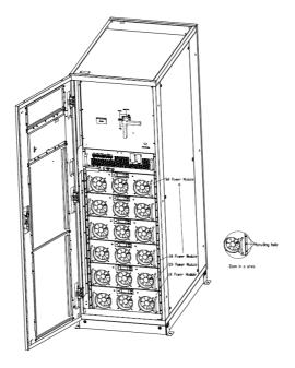
Figure 2-9 Installing power modules
