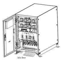
Figure 2-11 Cable Entry for 2-slot and 4-slot cabinets
