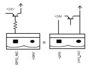
Figure 2-24 Diagram of input port for remote EPO Table 2-9 Description of input port for remote EPO
