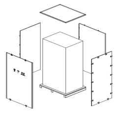
Figure 2-3 disassemble the case
