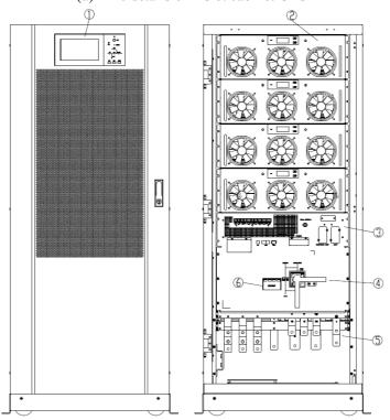
① Panel with color screen; ② Power module; ③ Bypass & monitoring unit (no hot-swappable function); ④ Breakers (input/bypass input/maintenance bypass/output); ⑤ Connection terminals; ⑥ SPD (optional)
