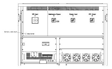
(e) Battery cold start button for 10-slot cabinet UPS Figure 4-1 the position of the battery cold start button
