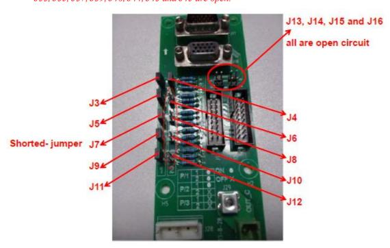
(b) The jumper setting for 6-slot and 10-slot cabinet UPS
