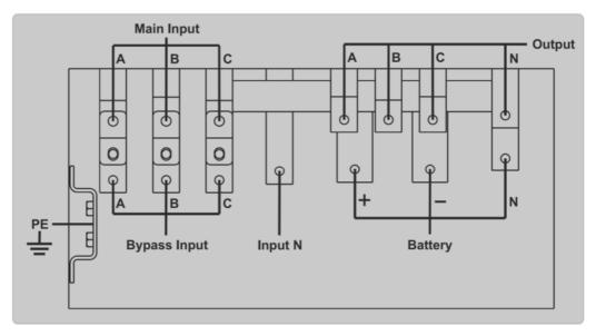
Figure 2-18 4-slot cabinet UPS connection terminals
