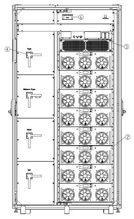
① Panel with color screen; ② Power module; ③ Bypass & monitoring module; ④ Manual bypass breaker; ⑤ Connection terminals; ⑥ SPD (optional)
