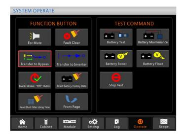
The operation interface for transferring to bypass
