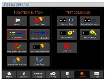
The operation interface for escaping bypass
