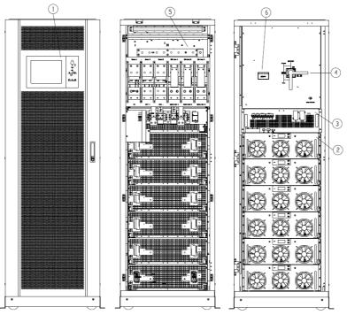
① Panel with color screen; ② Power module; ③ Bypass & monitoring module; ④ Manual bypass breaker; ⑤ Connection terminals; ⑥ SPD (optional)
