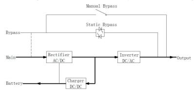
Figure 1-5 Normal mode operation diagram
