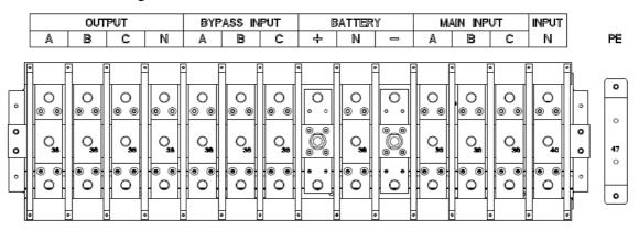
Figure 2-21 10-slot cabinet UPS connection terminals
