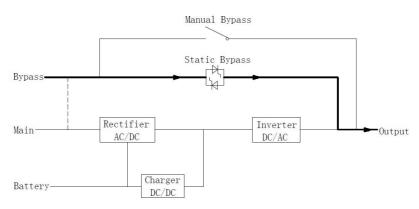
Figure 1-7 Bypass mode operation diagram
