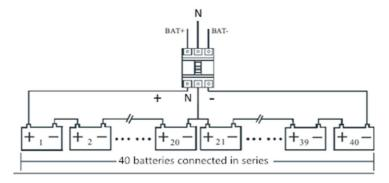
Figure 2-10 Battery string wiring diagram
