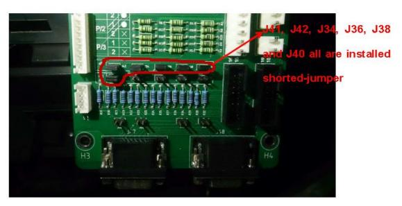
(a) The jumper setting for 2-slot and 4-slot cabinet UPS  $\,$
