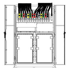
Figure 2-15 Cable Entry for 10-slot cabinet (Top Entry)
