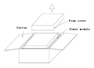
Figure 2-7 remove the foam cover
